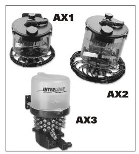
A geared synchronous motor connected to a camshaft mechanically activates a series of pumping units. A rotating impeller within the reservoir ensures an even flow of lubricant to these units. An integral PCB controls the delay period(s) and then initiates a complete revolution of the cam, thereby completing one lubrication cycle.
